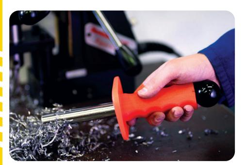
The Raptor swarf stick helps to keep your work place tidy. This handheld lightweight tool helps attract ferrous metal chippings and swarf to the stick which can then be easily removed.
