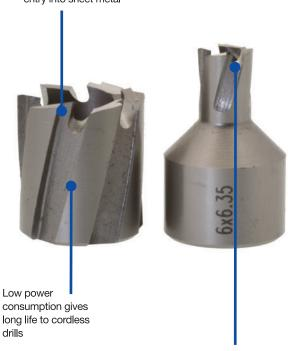
Annular cutting action requiring low thrust with less burring on exit
